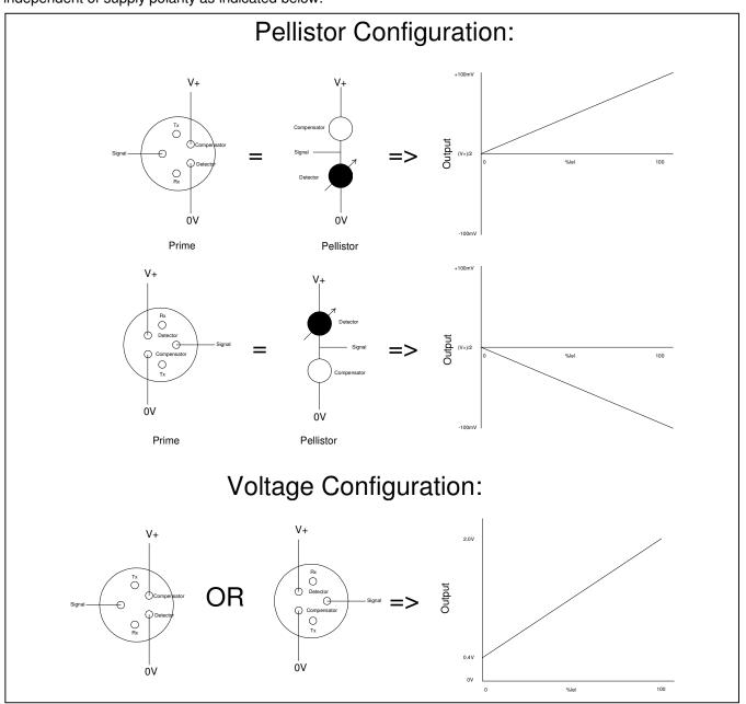
The Prime1 can be configured for a pellistor format output or a linear voltage output. Both output formats are independent of supply polarity as indicated below:
