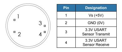
CONNECTION: Four gold-plated pins (0.64mm<sup>2</sup>) on a 2.54mm grid for PCB mounting via sockets or hand soldering using no-clean flux.
