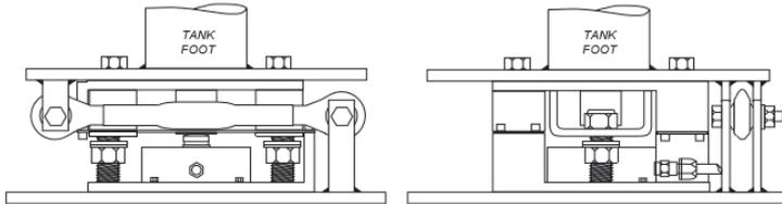
HORIZONTAL RESTRAINTS PLACEMENT ON 3/4 SUPPORTS: The restraining elements can be positioned both on supports and on the four sides, centrally between two supports.
