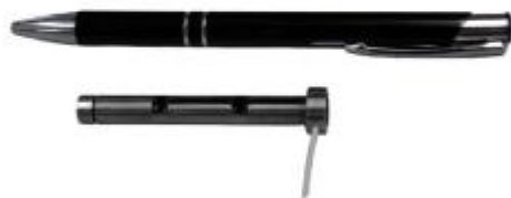
An externally strain gauged load pin.
