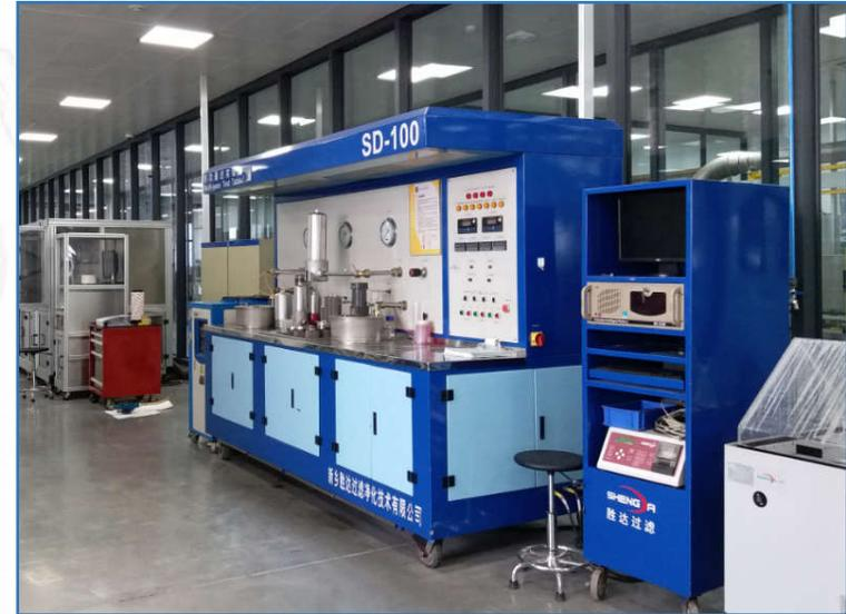
Flow resistance Test Rig
