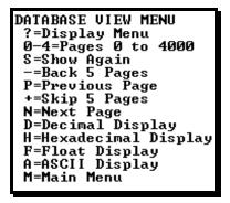
All data contained in the module's database is available for viewing using the commands. Refer to the Modbus Protocol Specification (page 157) for information on the structure of Modbus messages. Each option available on the menu is discussed in the following topics.
